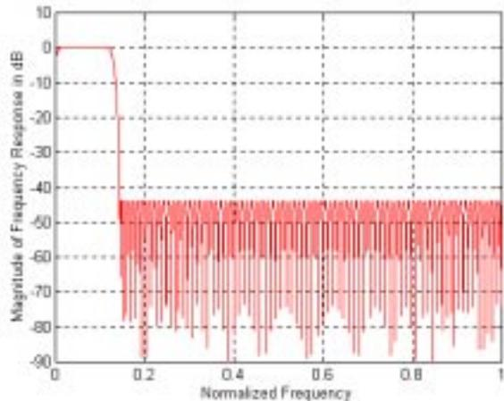
Fig. 4: The magnitude frequency response of the 8<sup>th</sup>-band equiripple stopband VSB filter used for calculating the polyphase components for the DFT polyphase filter banks in the example.
