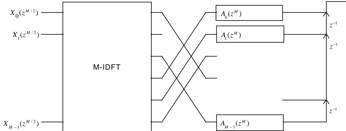
Fig. 5. Transmitter.  $M$  real input sequences are applied at rate  $2/M$  to an IFFT transformer, resulting in  $M$  complex sequences at rate  $2/M$ . These are then filtered by the  $M$  polyphase filters, and the output is obtained by summing the filter outputs properly. If  $M/2$  is even, then a further phasing is necessary at the input.
