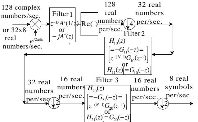
Note 1: The  $G_{10}(z)$  and  $G_{11}(z)$  are the lowpass and highpass transfer functions of the QMF pair next to the root of the synthesis filter bank trees, and the  $G_{20}(z)$  and  $G_{21}(z)$  are the transfer functions of the QMF pairs at the leaves of the trees.
