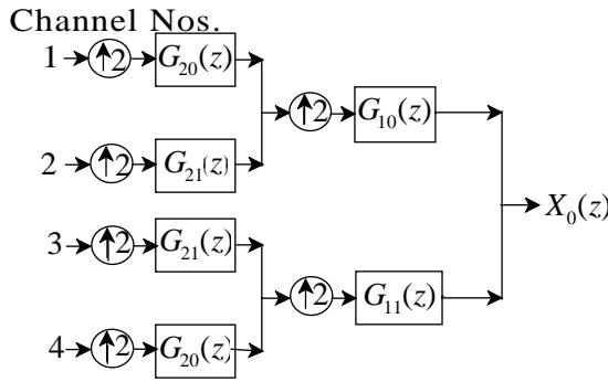
Fig. 1. The first basic 4-input wavelet packet-based synthesis filter bank repeated 3 times, with different channel numbering each time with successive output signals at the roots as the input signals  $X_1(z)$ ,  $X_2(z)$  and  $X_3(z)$  to a DFT polyphase synthesis filter bank shown in Fig. 2.
