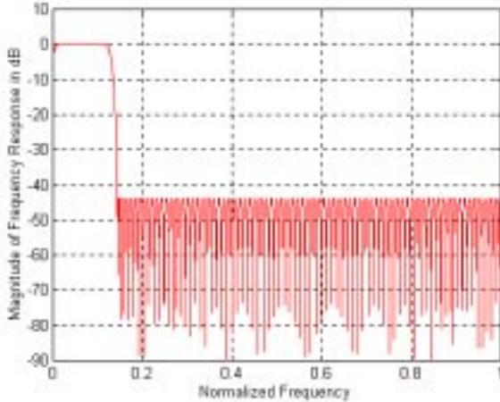
Fig. 4: The magnitude frequency response of the 8<sup>th</sup>-band equiripple stopband VSB filter used for calculating the polyphase components for the DFT polyphase filter banks in the example.
