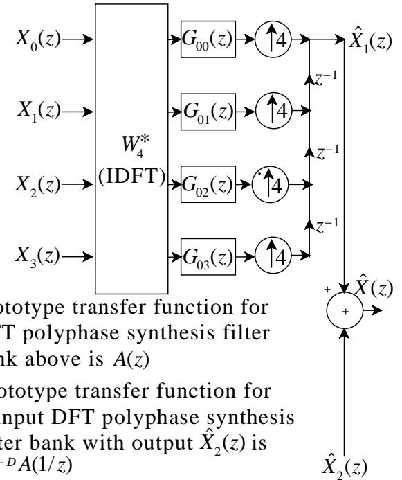
Fig. 2. Arrangement of DFT polyphase synthesis filter banks.
