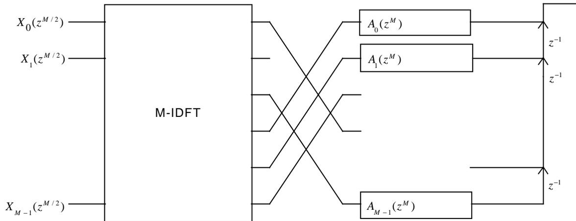
Fig. 5. Transmitter.  $M$  real input sequences are applied at rate  $2/M$  to an IDFT transformer, resulting in  $M$  complex sequences at rate  $2/M$ . These are then filtered by the  $M$  polyphase filters, and the output is obtained by summing the filter outputs properly. If  $M/2$  is even, then a further phasing is necessary at the input.
