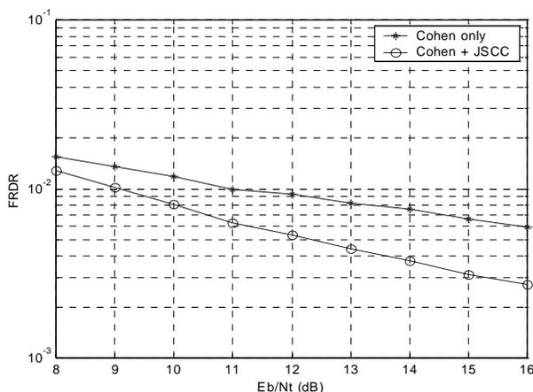
**Fig.4 FRDR of JSCC-RDA with Cohen's BRDA in the one-path Rayleigh fading channel**
