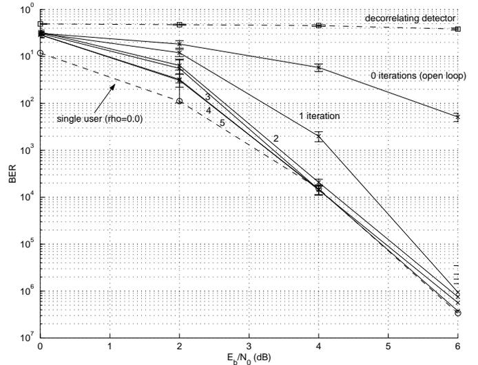
Fig. 3. Coded transmission over AWGN channel using  $r = \frac{1}{2}$  convolutional code, decorrelating detector and Moher's algorithm,  $\rho = 0.9$ , and  $K = 2$  users.
