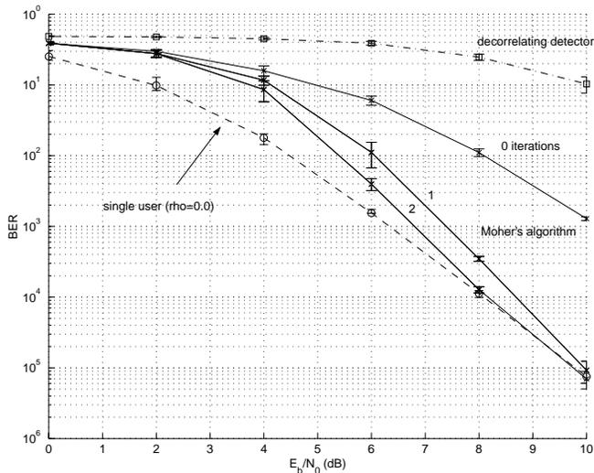
Fig. 4. Coded transmission over Rayleigh channel using  $r = \frac{1}{2}$  convolutional code, decorrelating detector and Moher's algorithm,  $K = 2$  users, and a crosscorrelation of  $\rho = 0.9$ .
