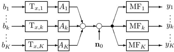
Fig. 1. Synchronous time discrete model for multiuser transmission over Rayleigh channel.
