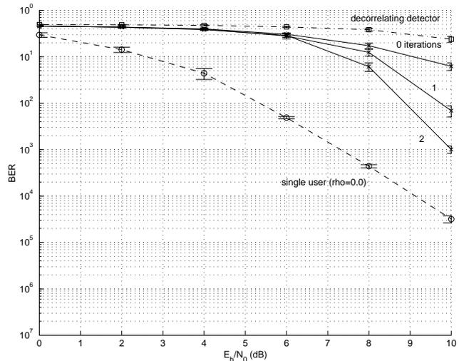
Fig. 5. Coded transmission over Rayleigh channel using  $r = \frac{1}{2}$  convolutional code, decorrelating detector and Moher's algorithm,  $K = 5$  users, and a crosscorrelation of  $\rho = 0.9$ .
