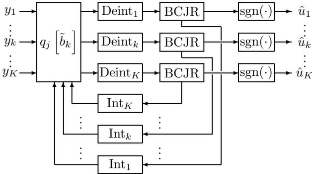
Fig. 2. Moher's multiuser detection algorithm in closed loop (iterative) mode.
