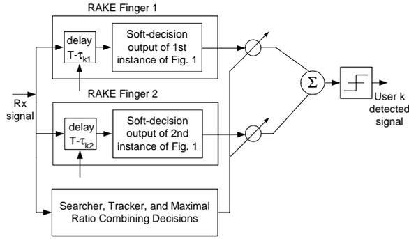
**Figure 2: RAKE Structure using the Improved Modified MMSE Detector**
