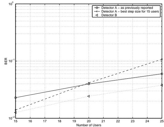
**Figure 3: BER of the Improved Modified MMSE Detector (detector B) vs. the Modified MMSE Detector of [5] (detector A)**
