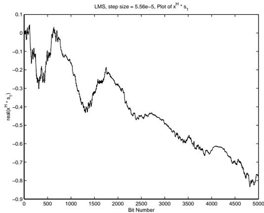
**Figure 4: Illustration of orthogonality problems without explicit orthogonal projection**
