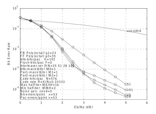
Fig. 1. Comparison of the BER performance for different block interleavers with 51, 25 and 28 columns and a dithered golden interleaver (101).
