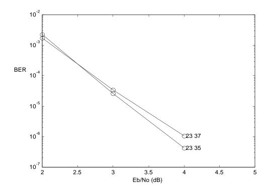
Fig. 2. Comparison of the BER performance for the BGM code and the (23, 35) code - N = 192, block interleaver with 128 columns, 2 iterations.
